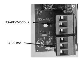
To prevent damage to the instrument, ensure that power is disconnected prior to making connections. For ease of connecting, remove the plug-in terminal block. Connections are labeled beside this termination on the PC board. The recommended cable is 22 AWG shielded twisted pair. The grey terminal block is removable to assist in making connections.
