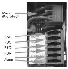
The CLX-XT will indicate the current status on another line called RSO or Remote Standby Output. These are a relay contact that is closed when busy (operating) and open when in standby mode.
