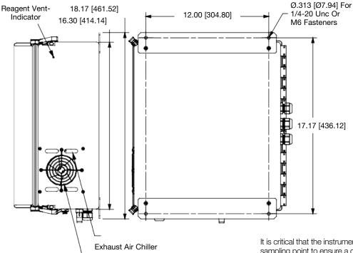
Figure 3: Overall Mounting Dimensions of the Instrument
