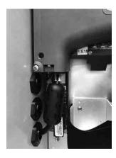
An optional connection is shown below. In this case the power to the measurement and cooler are made at this termination block. This termination will be located above the reagent cooling chamber.
